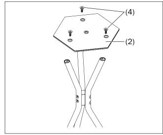
2. Screw the mounting plate (2) to the mounted support legs with three screws of type M4×10 (4). Do not overtighten these screws. Otherwise, the plastic threads in the support legs will be damaged.
