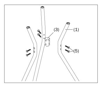
1. Screw the three support legs (1) to the connecting piece (3) using two screws of type M4×20 (5) each.
