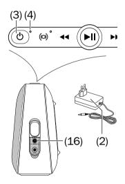
The integrated Li-lon rechargeable battery is charged as soon as the Motiv Go is supplied with power from the mains adapter (2) via the connection (16).
