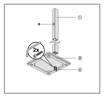
1. Use two cylinder head screws (a) to screw the tube (1) securely onto the base plate (8). Align the tube so that the bolt (a) is facing forward.
