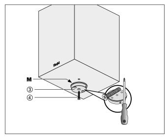
Screw the speaker bracket ③ on the speaker from below using the screw ④. The M mark must point to the front in the process.
