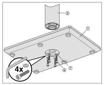
Screw the pipe ② on the base plate ① using four screws
