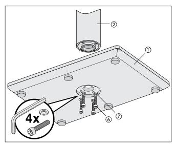
1. Screw the pipe (2) on the base plate (1) using four screws (6) and four washers (7). The big hole on the upper end is the cable feedthrough which should point to the back.
