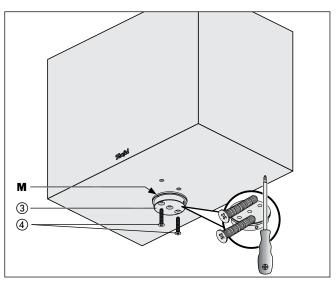
3. Screw the speaker bracket ③ on the speaker from below using two screws ④. The **M** mark must point to the front in the process.
