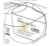
It indicates the battery level is between 21% to 45%. When charging, the LED breathes orange.
