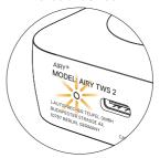
It indicates the battery level is between 21% to 45%. When charging, the LED breathes orange.
