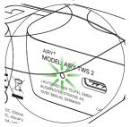
It indicates the battery level is over 71%. When charging,the LED breathes green.
