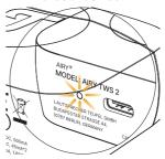
It indicates the battery level is between 21% to 45%. When charging,the LED breathes orange.
