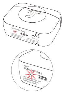
It indicates the battery level is below 20%. When charging, the LED breathes red.
