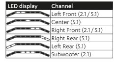
☑ Channel level mode has been activated and the volume can be set. for the selected channel.
