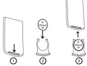
Inserting new batteries into the remote control
