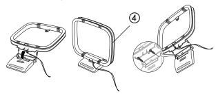
Connect the antenna cable with the jacks **14** "AM" on the back of the DVD receiver. Push down the lever on the terminal and run the cable end into the above opening. Releasing the lever will hold the cable in place.
