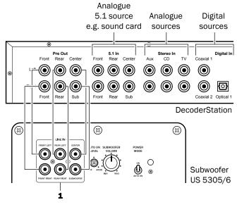
2. Connect the LINE IN jacks 1 of the subwoofer with the 5.1 output jacks of a preamplifier such as a decoder station using the included RCA cable.
