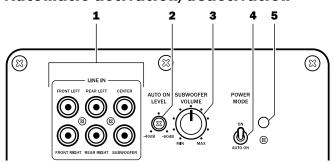
With the switch 4 "POWER MODE" you can switch the operating state:
