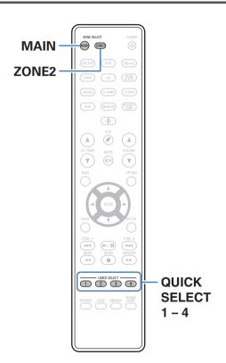
Settings such as the input source, volume level and sound mode can be registered to the QUICK SELECT 1 - 4 buttons.
