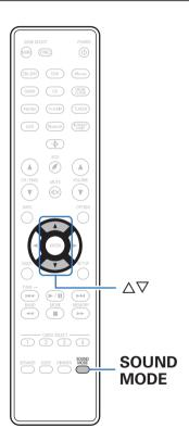
This unit has a selection of sound modes for you to enjoy: a Direct mode that plays audio exactly as it is recorded on the input source, a Stereo mode that adjusts the bass and treble output and a Pure Direct mode that enhances the quality of the audio that is played in Direct mode.
