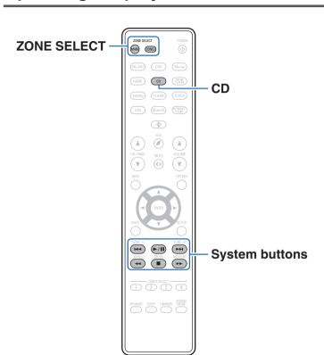
Press CD in the input source select buttons to operate your Denon CD player with the system control buttons.
