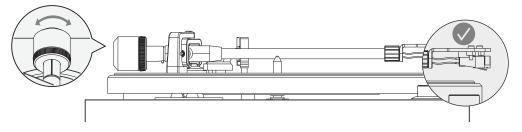
6. Set only the counterweight indicator ring to "0" on the center line while keeping the tonearm balanced then lock the tonearm on the tonearm rest.
