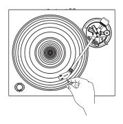
4. Hold the headshell and lower the cueing lever completely. Be careful not to let the stylus touch the platter.
