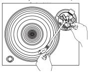
5. With the cueing lever now lowered, turn the entire counterweight until the tonearm is balanced and floating horizontally when headshell is released.
