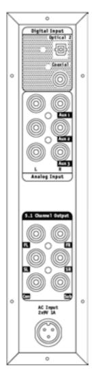
Specification of the connections on the back of the decoderstation 3 and their functions.
