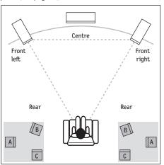
Make sure that the centre speaker and the two front speakers are positioned in a straight line, or on a slight arc with the TV/screen. If the distances between you and the speakers vary significantly, this will degrade the audio signal's spatial imaging. Make sure to align your speakers properly so they sound as good as possible.
