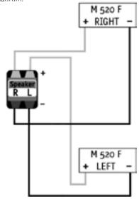
First, you need to connect the ends of your speaker cables to the L/R speaker outputs of your amplifier/receiver and to the "High Level" speaker terminals of the two column speakers.
