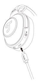
Use the enclosed type-c cable to connect the USB-C port **3** of the headphones with a USB port on a PC or a USB power adapter.
