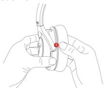
Please hold the auricle firmly with one hand (1) during the change, as the swivel joint could break if too much pressure is applied.
