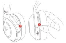
Start at the top of the cushion (2) and then go between the cushion and the headset, for example, with the thumb nail of your thumb. In this way you can remove the cushion step by step.
