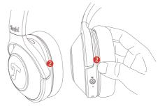
Start at the top of the cushion (2) and then go between the cushion and the headset, for example, with the thumb nail of your thumb. In this way you can remove the cushion step by step.
