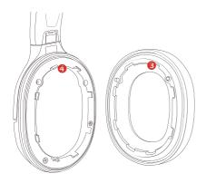
Please be careful not to make any twisting movements, as the protrusion inside the headset could possibly be damaged.
