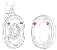
As shown above, there are 8 plastic edges and 2 grooves (3), please slide the cushion under 2-4 plastic edges and aim the protrusions (4) to the grooves, then go around the cushion, click in the rest.
