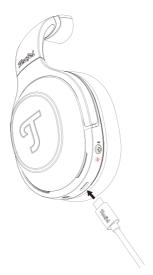
Use the enclosed type-c cable to connect the USB-C port **4** of the headphones with a USB port on a PC or a USB power adapter. During charging, the status LED is pulsing in yellow. When the headphones are fully charged, the status LED lights up in white and will fade out after 1 minute.
