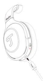
Use the enclosed type-c cable to connect the USB-C port **4** of the headphones with a USB port on a PC or a USB power adapter. During charging, the status LED is pulsing in yellow. When the headphones are fully charged, the status LED lights up in white and will fade out after 1 minute.
