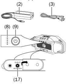
Four white LEDs on the rechargeable battery indicator **(8)** signalise the charging process:
