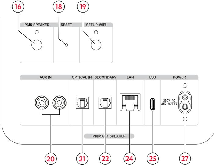
Connections and buttons on the primary loudspeaker
