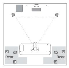
The rear speakers are set up or hung to the side of or behind the listener at a height of 1.20 m to 2.10 m (see the grey areas in the graphic).
