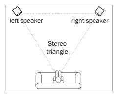
The speakers should be situated to the left and right of the listener and if possible, form an equilateral triangle with the listener – the so-called stereo triangle (distance from the listener = distance between the speakers). The speakers should project sound straight into the room or be arranged slightly towards the listener.
