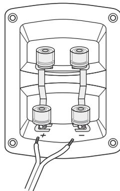
The contact bridges between the connector terminals must not be removed; you can connect the speaker cables accordingly to the top or bottom terminals.
