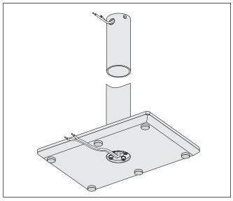
2. Run the speaker cable through the upper hole and through the pipe until it extends somewhat out of the opening in the base plate. Then pull it through until there is sufficient length left for connecting the speaker at the top.
