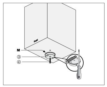
3. Screw the speaker bracket ③ on the speaker from below using the screw ④. The **M** mark must point to the front in the process.
