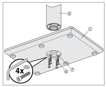
1. Screw the pipe ② on the base plate ① using four screws ⑥ and four washers ⑦. The big hole on the upper end is the cable feedthrough which should point to the back.
