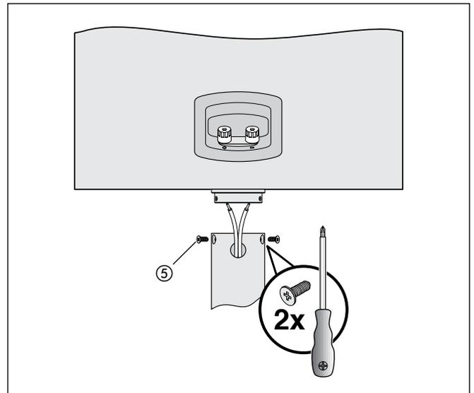
4. Place the speaker with the speaker bracket on the pipe and screw the bracket on the pipe through the bore holes using two screws ⑤.
