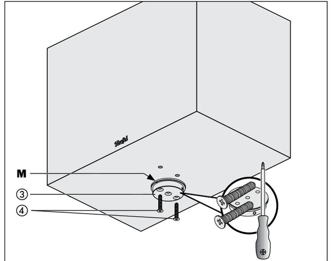
3. Screw the speaker bracket ③ on the speaker from below using two screws ④. The **M** mark must point to the front in the process.
