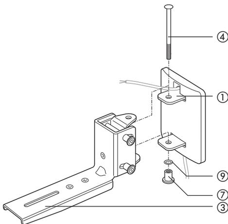
10. Tighten the carriage bolt ④ with the washer ⑨ and the nut ⑦.
