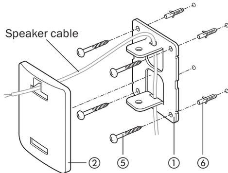
6. Screw the base plate ① on the wall using four half round head screws ⑤.
