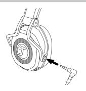
Connect the 3.5 mm jack plug output of the headphones and the headphone jack of your audio system or your smartphone using the enclosed connector cable.
