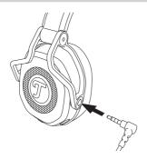
Connect the 3.5 mm jack plug output of the headphones and the headphone jack of your audio system or your smartphone using the enclosed connector cable.
