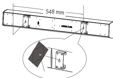
Each side of the bracket is attached to the wall using a screw.
