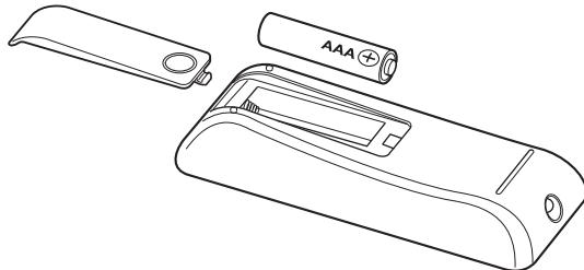
To change the battery, remove the battery compartment cover from the remote control, change the battery and put the cover back in place.
