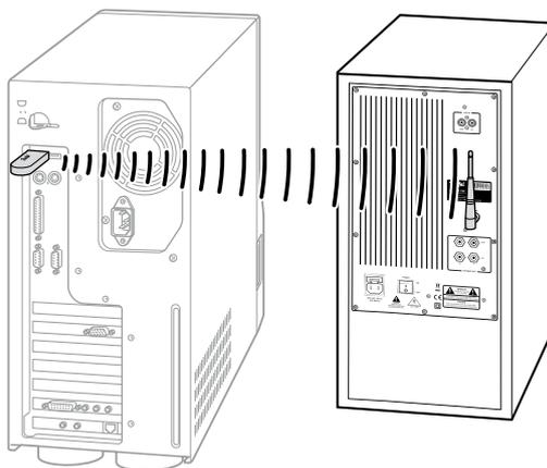
To use the soundcard, screw the antenna **6** onto the jack **5** "ANTENNA".
