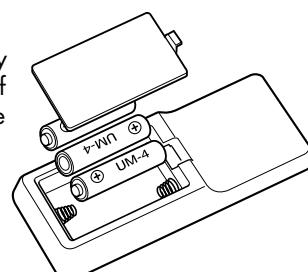
Insert the batteries in the battery compartment as shown in the figure. Put the cover back on the compartment and push it closed.
