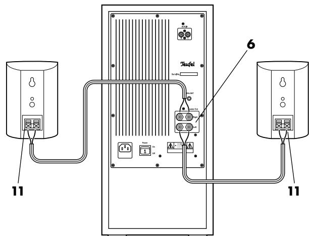
The connector terminals **6** "SPEAKER OUT" for the right ("Right") and left ("Left") speakers are located on the back of the subwoofer.
