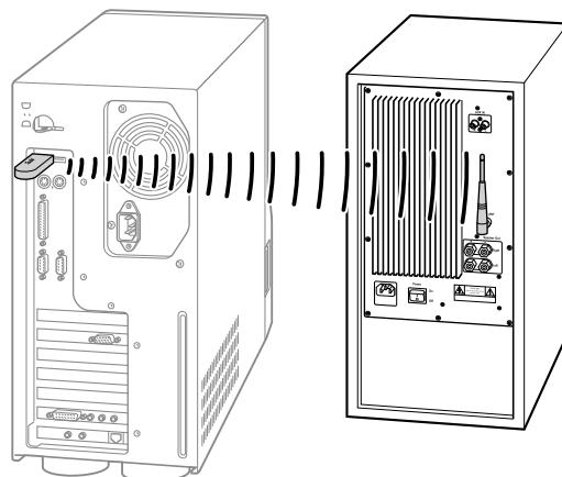
To use the soundcard, screw the antenna **6** onto the jack **5** "2.4 GHz ANT".
