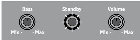
Press the »Standby« button to switch on the device fully – the rings encircling each of the three control elements turn »blue« indicating the subwoofer is now ready for use.
