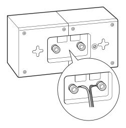
On the back of the speakers are the connection terminals, with 2 terminal clips. You can connect the speaker cables here directly or with banana plugs or spade terminals from our catalogue. The terminals are marked in red (+) and black(-).
