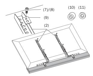
11. First hang the TV-set with the TV rails on the top of the base plate and carefully press along the bottom until the mount audibly clicks into place.
