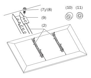
15. First hang the TV-set with the TV rails on the top of the base plate and carefully press along the bottom until the mount audibly clicks into place.
