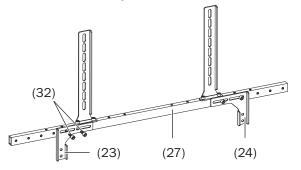
Mount the soundbar on the L-brackets (23)/(24) or (25)/(26). Depending on the soundbar, use either the locking screws (29) or the holding screws (31) with the lock nuts (30). Also use the washers (28) if necessary.
