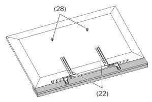
Screw the two TV rails (2) onto the support rails
