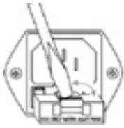
If the Power LED on the rear panel does not light up, replace the fuse with a fuse of equal rating (see page 14, ⑧).
