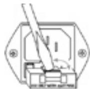
If the Power LED on the rear panel does not light up, replace the fuse with a fuse of equal rating (see page 14, point 5).
