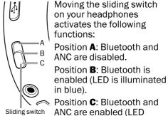
If you have connected the headphones via a cable, you can activate the ANC function by moving the sliding switch to position **C**.
