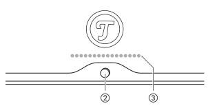
• By turning the control dial (2) clockwise, you can switch the MD16 on and increase the volume at the same time.
