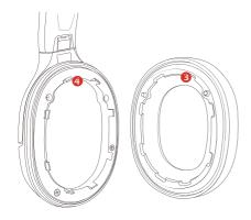
Please be careful not to make any twisting movements, as the protrusion inside the headset could possibly be damaged.
