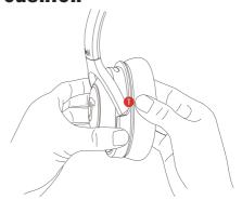
Please hold the auricle firmly with one hand (1) during the change, as the swivel joint could break if too much pressure is applied.
