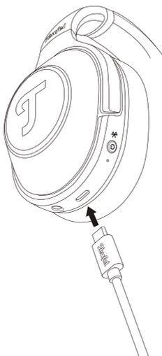
Use the enclosed type-c cable to connect the USB-C port **3** of the headphones with a USB port on a PC or a USB power adapter.
