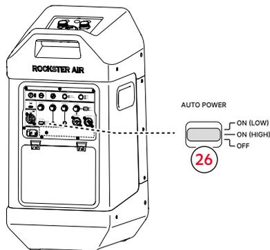
Depending on the operating mode and the selected setting, the speaker switches off after a few minutes without an input signal or switches to network standby mode.
