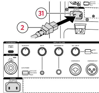
1. Connect the mains cable (2) to the speaker power socket (31).
