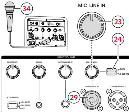
1. Connect a microphone (34) to the COMPANION IN socket (29).
