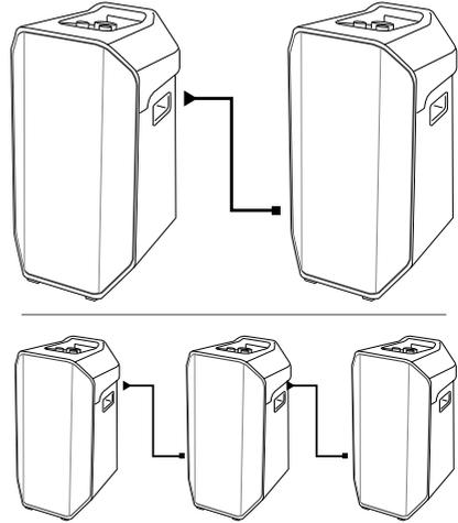
Via COMPANION IN (29) and COMPANION OUT (30) multiple speakers can be connected together in Master-Companion mode.
