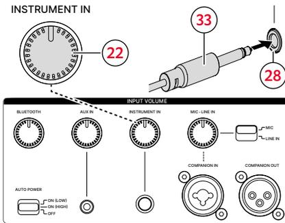
1. Connect the instrument (33) to the INSTRUMENT IN socket (28) using a mono cable with a 6.3 mm jack plug.
