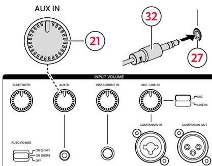
1. Connect the external player (32) to the AUX socket (27) using a stereo cable with a 3.5 mm jack plug.
