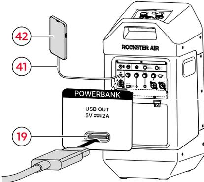
1. Connect the USB-C cable (41) to the USB-C port (19).
