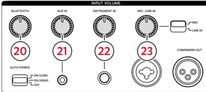
The volume is set via the Master volume controller (13) and the Input volume-controller of the input sources (20-23).
