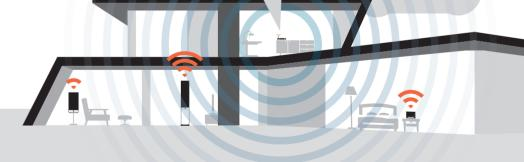
During the setup process, it is important to ensure that all Raumfeld devices receive a sufficient Wi-Fi signal. A signal that is too weak can lead to dropped connections.
