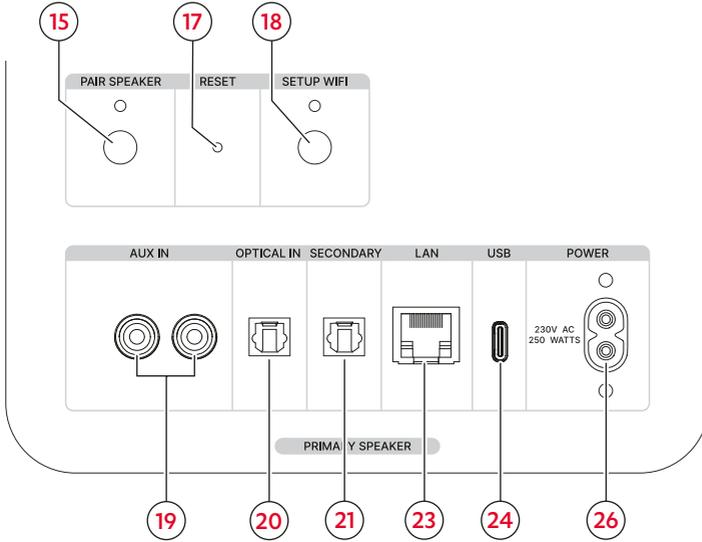
Connections and buttons on the primary loudspeaker
