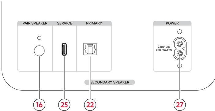
Connections and buttons on the secondary loudspeaker
