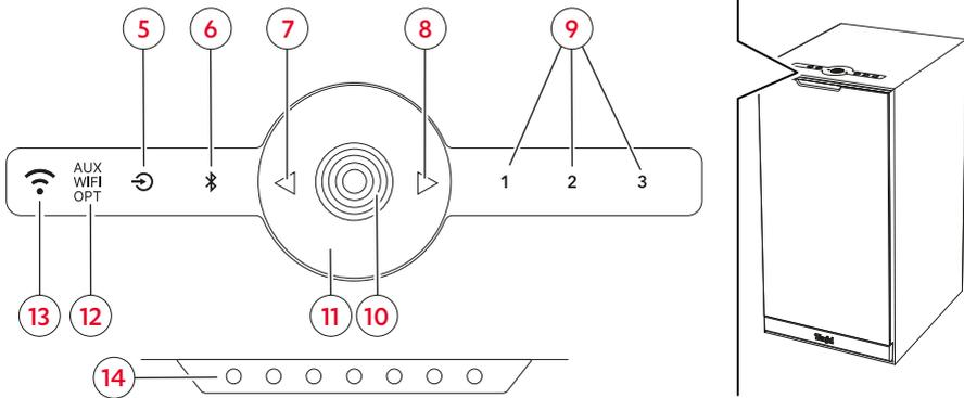
Operating panel and status LEDs on the primary loudspeaker
