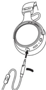
1. The enclosed connector cable has two 3.5 mm jack plugs. Insert the notched 3.5 mm jack plug into the 3.5 mm jack **5** of the headphones. Make sure the cable remote control is closer to the headphones than to your audio system or smartphone.
