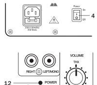
• Use mains switch 4 "Power" to switch the main power supply on or off. When the subwoofer is activated, the power LED 12 "Power" is green. If the subwoofer is in standby, it is red.
