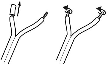
2. Turn the connector terminal counterclockwise until loose. Run the stripped cable end into the hole that is now visible. Turn the terminal clockwise until closed. The cable has now been clamped into place.
