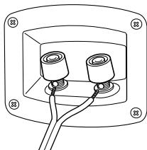
3. Connect the other end of the speaker cable to the front speaker outputs of your amplifier. You can find notes on this in the corresponding operating instructions.
